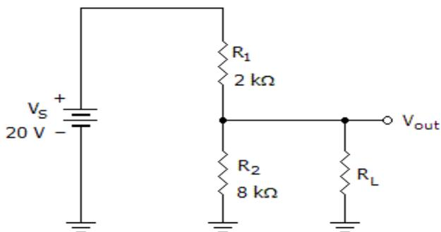
If the load in the given circuit is  $120 \text{ k}$  , what is the loaded output voltage?
