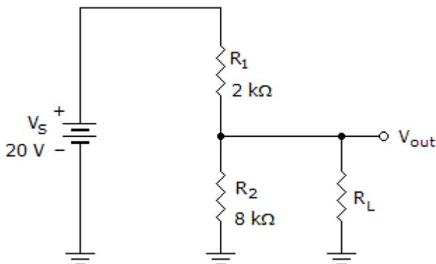
If the load in the given circuit is  $80\text{ k}\Omega$ , what is the **bleeder current**?
